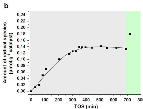
Fig. 4. CW-EPR spectra at various TOS (a) and amount of radical species (b) for the HZSM-5(40) fresh catalyst (from 0 to 720 min).
