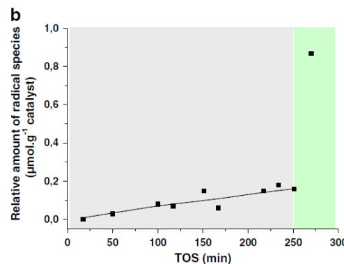
Fig. 5. CW-EPR spectra at various TOS (a) and relative amount of radical species (b) for the HZSM-5(40) coked catalyst (from 0 to 270 min).
