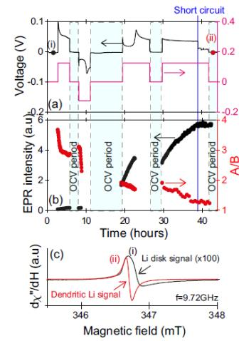
CW-EPR spectra of the Li//Li symmetric battery at different polarization stages, together with the electrochemical profile
