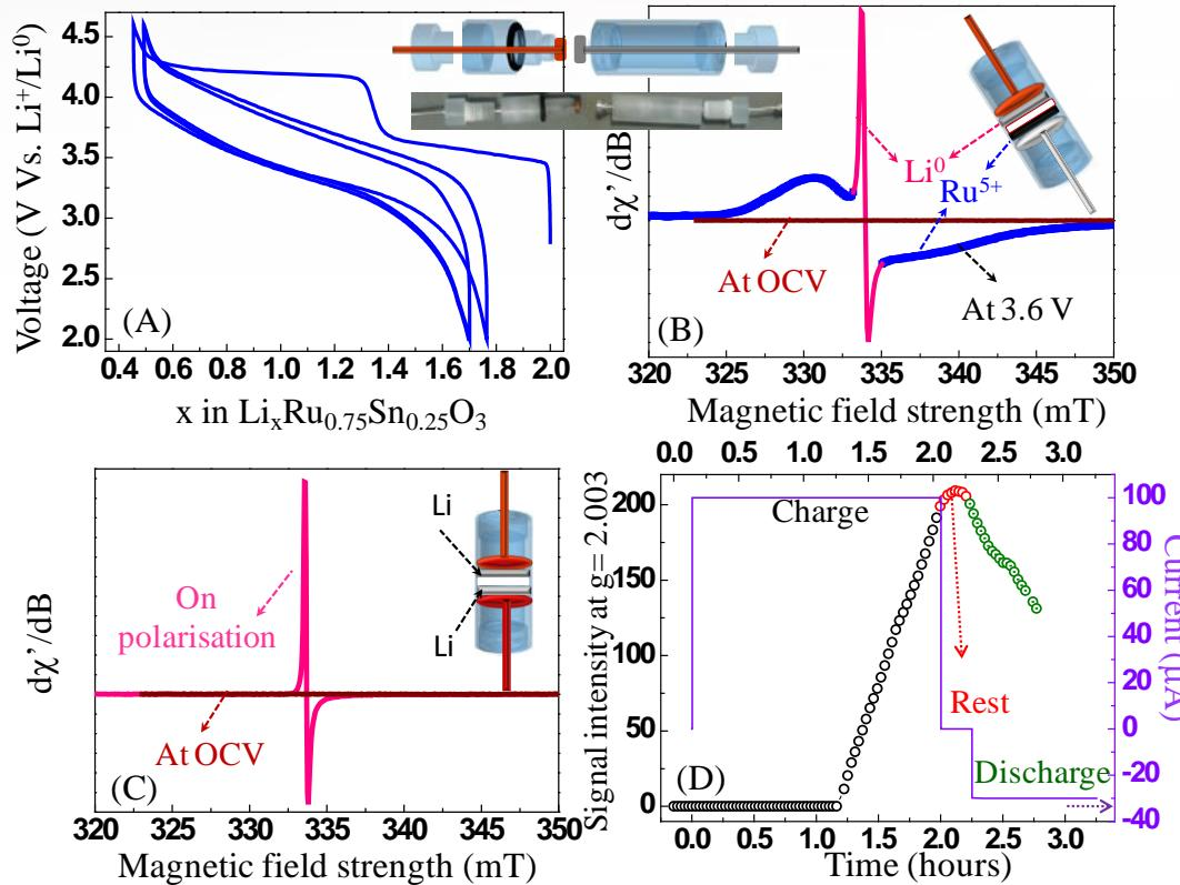
Sathiya, M., Leriche, J.-B., Salager, E., Gourier, D., Tarascon, J.-M., & Vezin, H. (2015). Electron paramagnetic resonance imaging for real-time monitoring of Li-ion batteries. *Nature Communications*, 6, 6276.
