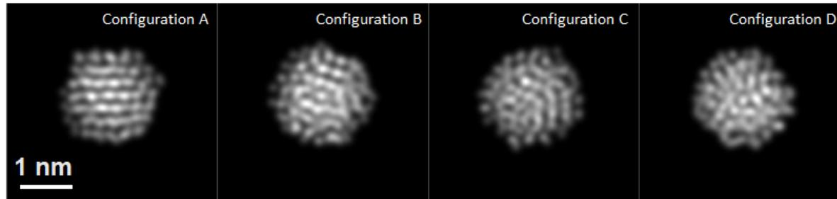
Structure evolution of Toh-Au<sub>201</sub>H<sub>122</sub> // [110] zone axis during MD simulations
