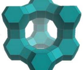
A hydrothermal treatment is generally performed for enhancing these properties by introducing a hierarchical porosity. Through the removal of framework Al, the structure rearranges for accommodating mesopores and hydrothermally stabilizes.
