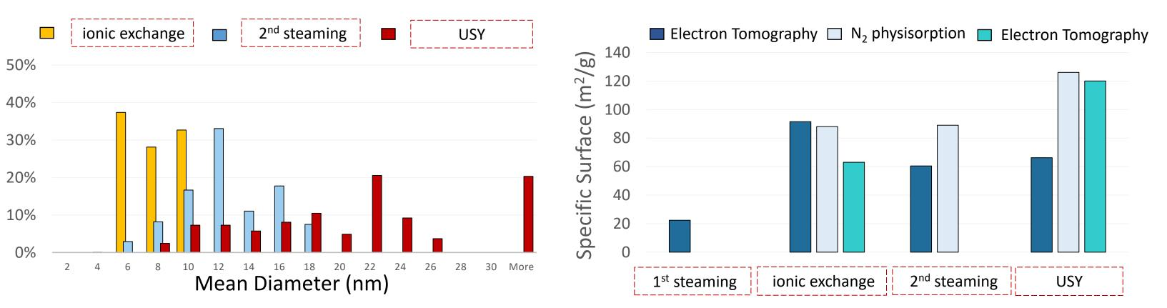
During the dealumination an increasing trend in the mesoporous volume, specific surface and mesoporous diameter, in agreement with the literature and with the correlated N<sub>2</sub> – physisorption analysis
